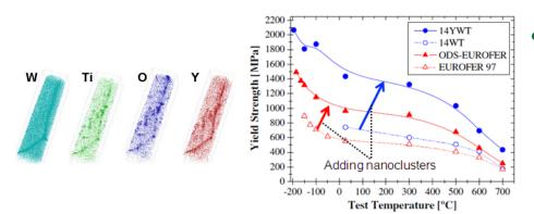
Stable nanoclusters (~2-4 nm in size) are found in ferritic alloys prepared by mechanical alloying and serve to increase strength even after long times at high temperatures
