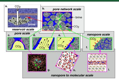
OBJECTIVES are to (1) develop molecular, nano-scale, and pore network scale approaches for controlling flow, dissolution, and precipitation in subsurface rock formations during emplacement of supercritical CO<sub>2</sub>; and (2) achieve a new level of prediction of long-term performance
