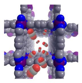
This EFRC will develop new strategies and materials that allow for energy efficient selective capture or separation of  $CO_2$  from gas mixtures based on molecule-specific chemical interactions.
