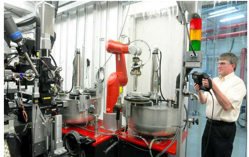
Robotic automation experimental set up for Synchrotron Protein Crystallography
