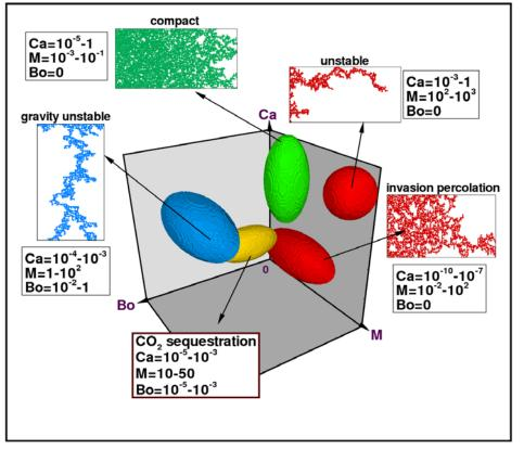
Map of microscopic drainage behavior in the parameter space of  $Ca_i M_i Bo_i$
