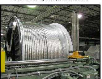
Toroidal field cable produced at New England Wire Technologies (Lisbon, NH)
