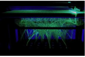
Figure 14 The WLS fiber detector, in daylight (left) and dark (right). The flat scintillator has an area of  $77 \times 38$  cm<sup>2</sup>, and scintillation light is coupled by 308 and 152 fibers feeding 25 and 7 photomultipliers, respectively, for the X and Y axes.
