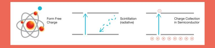
In each of these cases, a certain energy,  $\eta$ , is required to create those secondary quanta, so that  $N = E_e / \eta$  secondary quanta are created. If the X-ray was photoelectrically absorbed, in which case  $E_e = E_{\gamma i}$  then a measurement of N is a measurement of the X-ray's energy.
