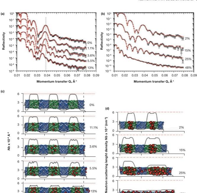
Distance from the substrate, Å Distance from the substrate, nm Figure 25 (a,b) Reflectivity profiles of symmetric (PS-d-b-PBMA) copolymer multilayers with different concentrations of small nanoparticles in (c) and big nanoparticles in (d). The volume fraction of nanoparticles is indicated in percent.
