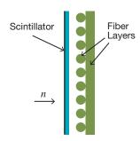
that absorbs the blue photons from the scintillator and re-emits the photons at a longer (green) wavelength (hence the name "wavelength-shifting"), some of which then travel to the ends of the fibers.
