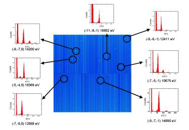
Figure 7 White light microdiffraction at ALS BL 12.3.2 with Berkeley Lab FastCCD.
