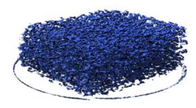
**Figure 28** 3-D Li distribution ( $\text{Li}_2\text{O}_2$ ) in coarser foam matrix, which can help to address interfacial transport and the Li transport in complex electrodes (degradation issues).
