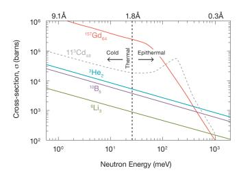
**Figure 12** Neutron absorption cross section vs. neutron energy.
