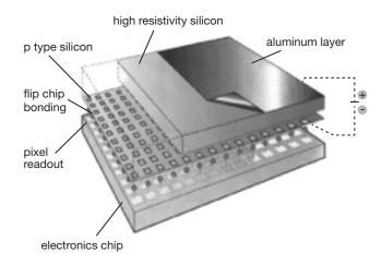
Figure 30 Hybrid pixel detector.
