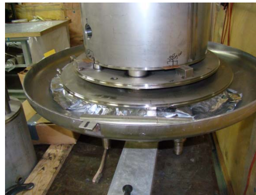
Cryostat Thermal Insulation
