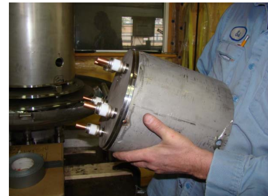
Sample Holder Housing with Current Leads Feedthrough
