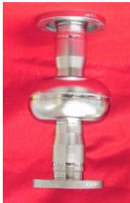
Single crystal Niobium gives promise for high gradients for acceleration (ILC)
