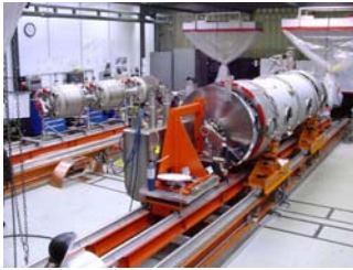
SNS SC RF cavities at JLAB
