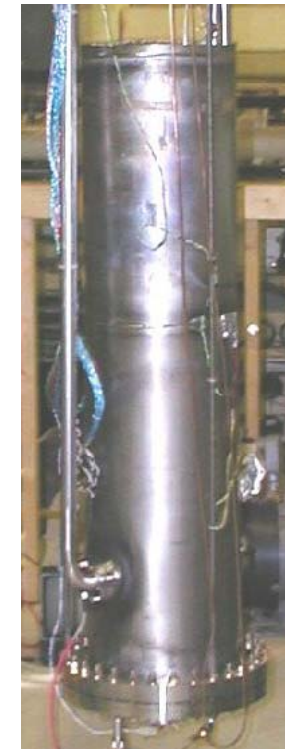
80.5 MHz Quarter-Wave resonator
