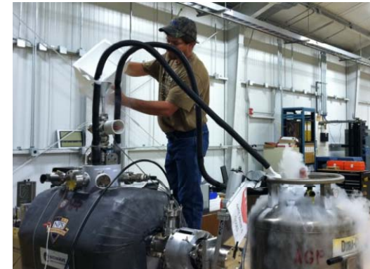
Batch filling with a 250L helium Dewar
