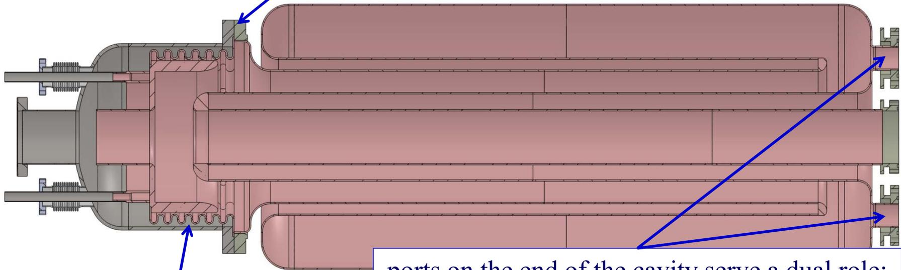
mechanical tuner motion with a Nb bellows which confines the fields (prevents power dissipation in the vacuum vessel)
