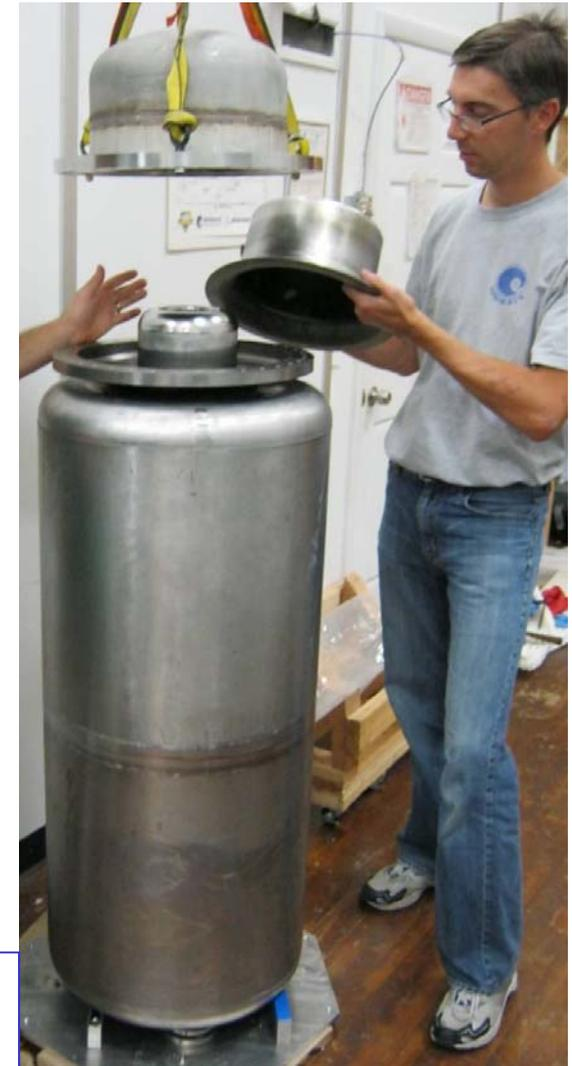
test fitting of all subassemblies prior to electron beam welding
