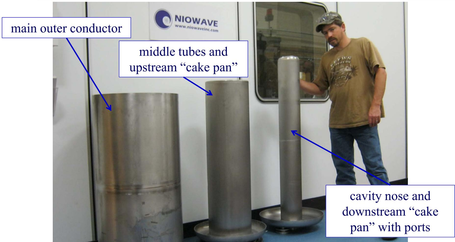
The large subassemblies are now ready to be joined (by electron beam welding) to create the main cavity.
