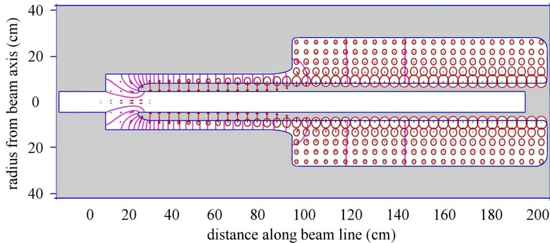
conventional quarter-wave structure with large capacitance to operate at 28 MHz
