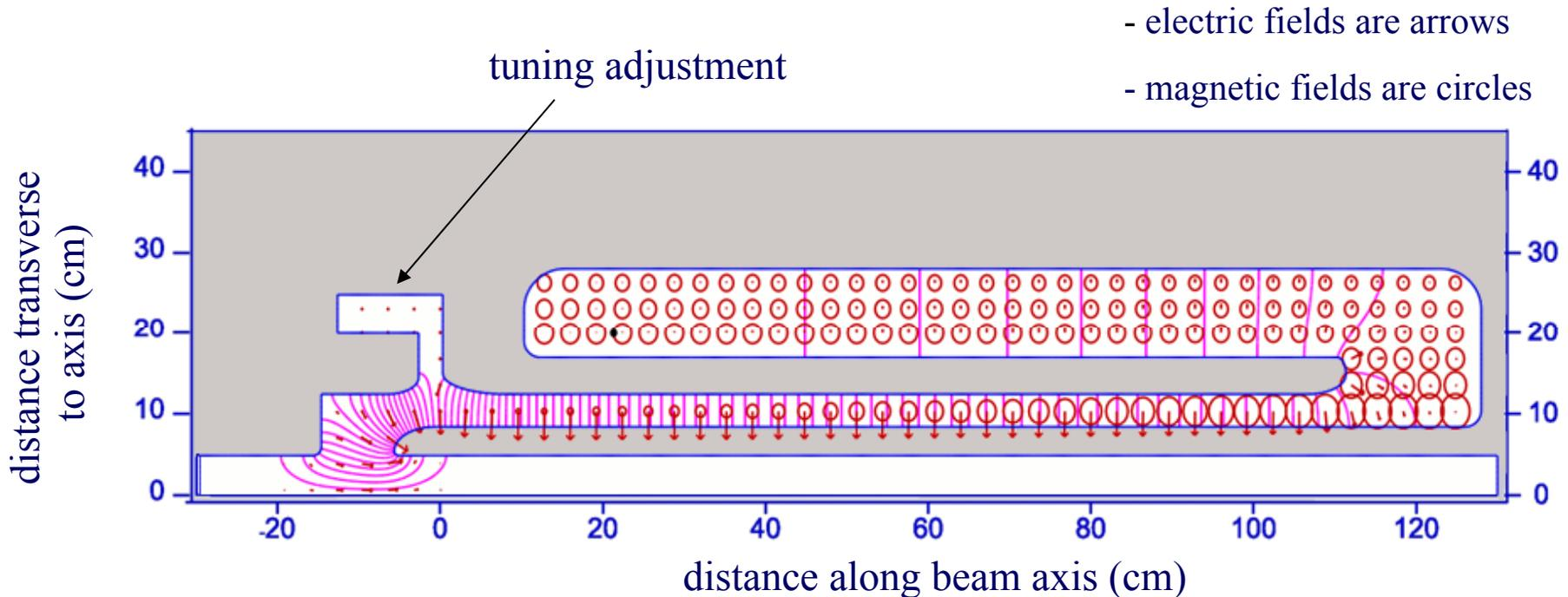
Addition of a second capacitor – only a small section must be moved to tune the cavity the required 200 kHz.
