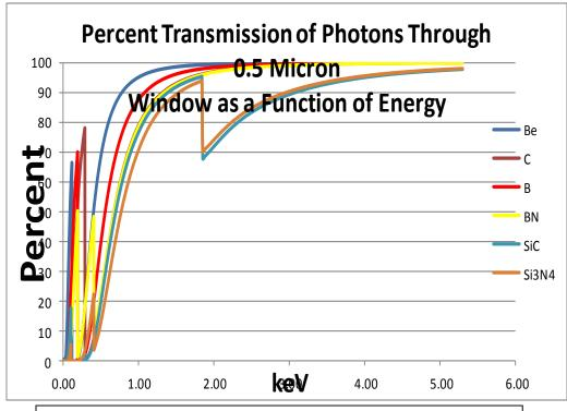
**Figure 2**: Calculated x-ray transmission curves for 0.5micron thick films of various materials at UHV. Please note that even though 0.5 micron thick Be has the best transmission, films/foils thinner than 8 microns cannot be used due to pin-holes and poor strength, which is why we need ceramic films.
