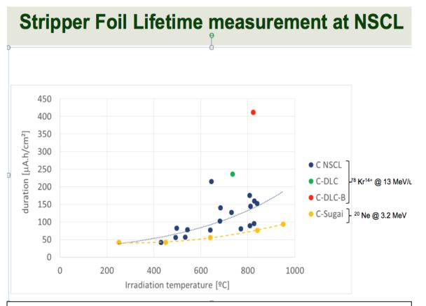
**Figure 10**: Lifetime result at the stripper injection system of the NSCL. The results are compared to results from Sugai with a Ne beam (I.Sugai et al., NIM B 269 (2011) 223)
