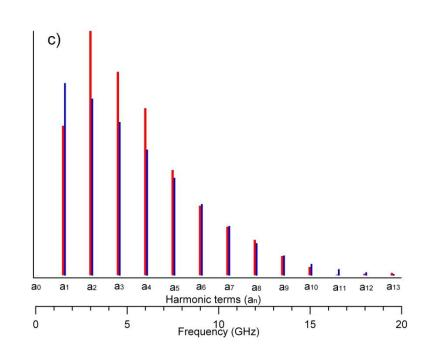
The ratio of these two series is the harmonic cavities transfer function. Once determined, the cavities transfer function can be used to un-distort subsequent data independent of new bunch shapes.
