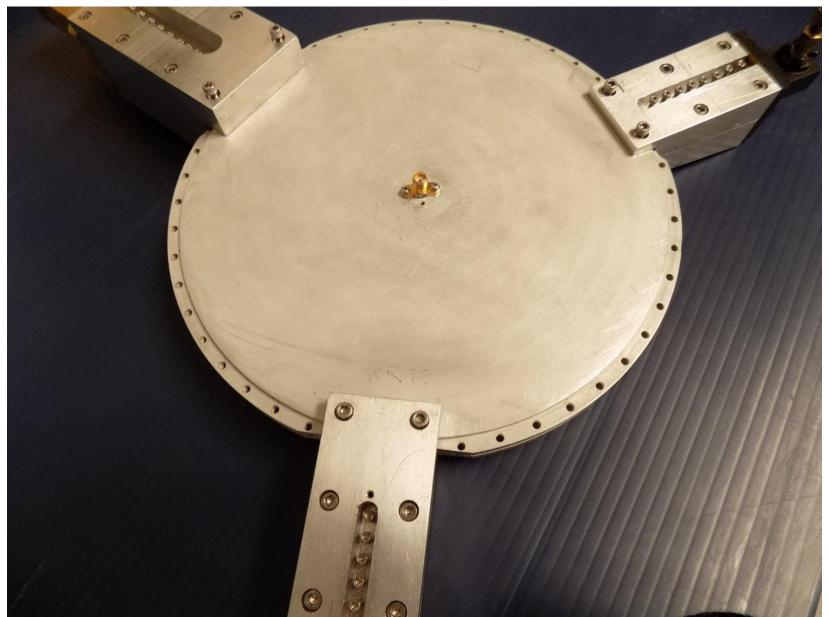
CNC Lathe/Mill hybrid can now machine harmonic cavities up to 8 ft. in diameter.
