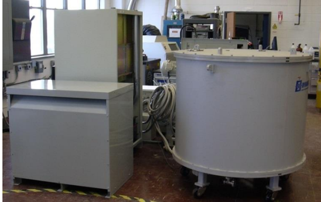
Conduction cooled cryostat at Ohio State University for testing both inductive and resistive SFCL coils
