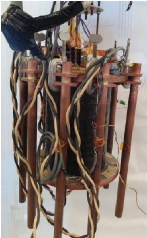
Coil dewar internal assembly
