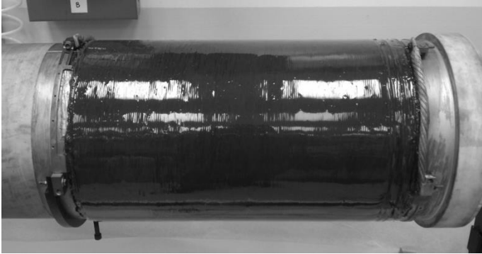
Coil for resistive SFCL
