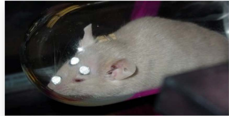
Three IR markers attached to the head of a mouse enable the AwakeSPECT system to obtain detailed, functional images of the brain of a conscious mouse as it moves around inside a clear burrow.
