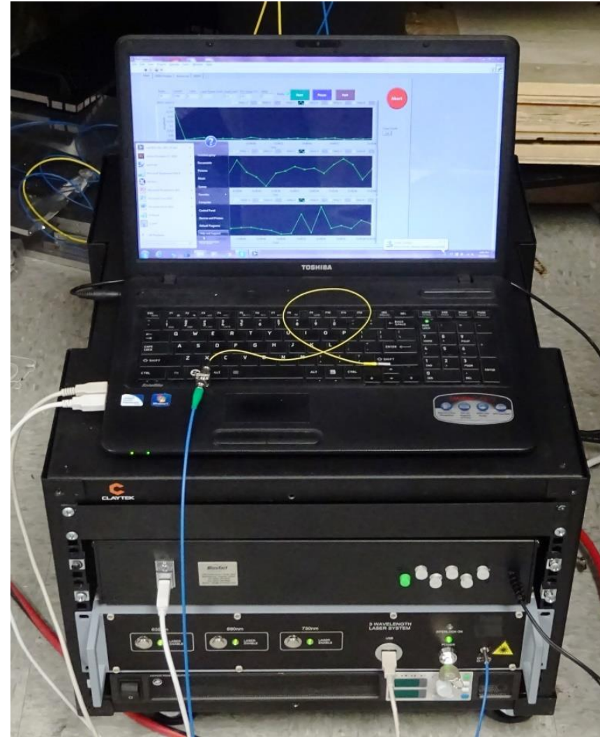
Stand-alone system prototype for interrogation of up to 3 sensors
