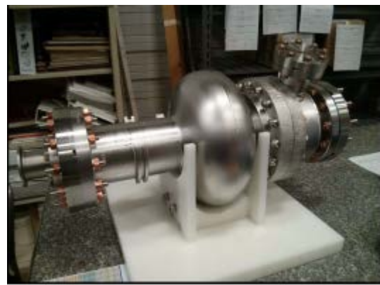
Compact, detachable coaxial coupler for SRF cavity (joint project with FNAL)
