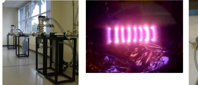
Need glow-discharge cleaning before Cu deposition, RF properties (at cryogenic temperatures) still to be determined
