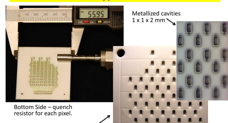
Top Cavity Side with metal vias and gas channel
