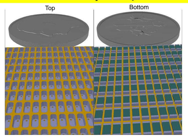
Microcavity-PPS prototype for 2015 (*dime coins for scale*): (Left) cavities with vias. (Right) surface-mount pixel resistors.
