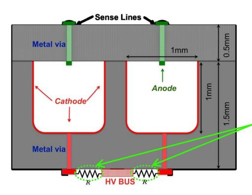
Closed gas cell individually quenched by an external resistor
