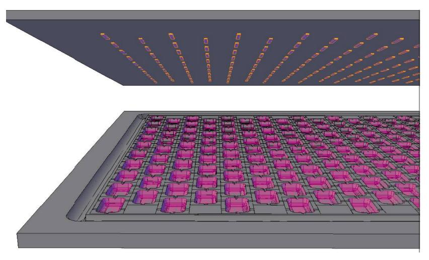
Perspective view of a pixel array with gas channels. Metallized cathode cavities on bottom plate with *vias* to HV bus. Anodes on top plate.
