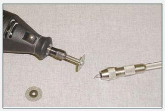
Method to Open Ampule in Hot Cell
