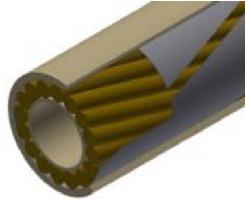
cutaway showing foil over-wrap
