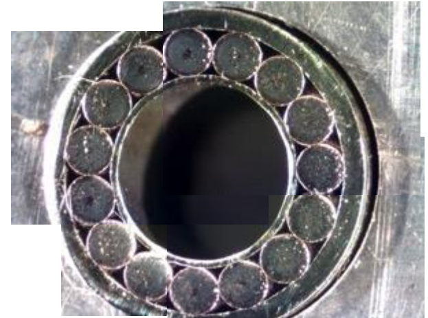
Cross section showing NbTi strands
