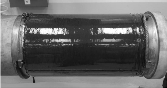
Coil for resistive SFCL
