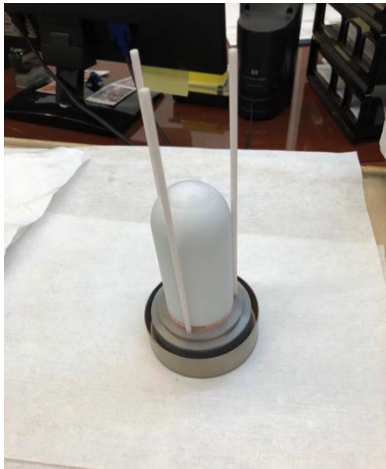
Window braze fixturing, (needed some rework)
