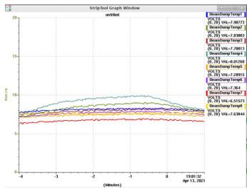
Thermal couples register beam induced temperature rise at the dump
