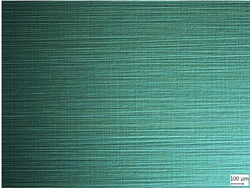
10 μm/hr 650°C Growth Temp with no Superlattice With a 2° (110) offcut on GaAs
