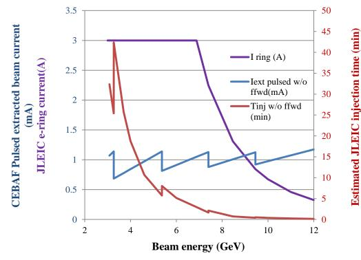
Assumes maximum kicker repetition rate 60 Hz Assumes head-tail energy droop of 0.2% (1/2 of the ±0.2% arc acceptance), no damping wiggler
