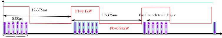
If ~0.2% droop is allowed, the estimated extraction beam current will be ~2mA at various energy, depending on cavity coupling and microphonics.
