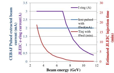
Estimated JLEIC pulsed injection current and injection time (limited by injector current only) with RF feedforward and varying number of passes
