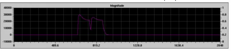
M56 measured beam current with laser A/C set to  $150\mu$ A (saturated)
