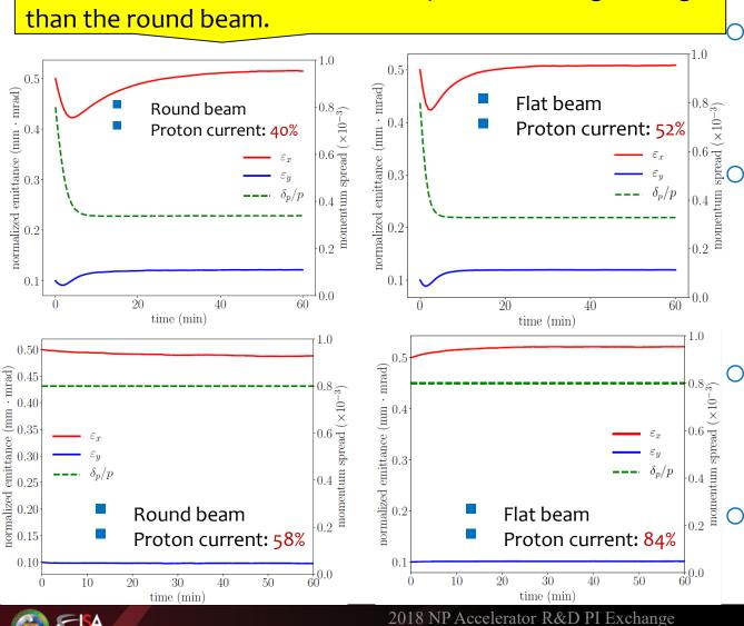
Flat beam with the same emittance provides strong cooling
