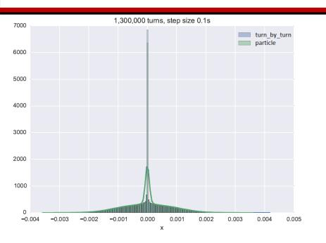
$\bigcirc$  dt = 0.1s, results are almost identical.  $\bigcirc$  dt = 0.5 s, the deviation starts to show, but not large.  $\bigcirc$  dt = 1s, the deviation becomes larger.
