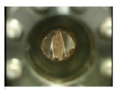
A thin film of liquid lithium  $\sim 420~\mu g/cm^2$  thick movies at  $\sim 70$  meters per second from the top to the bottom of the opening. A beam of Uranium Ions will be passed through the film to strip away atomic electrons so that the uranium ions can be accelerated to the full energy of the FRIB .
