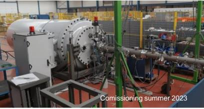
Nuclear Astrophysics: LENA Upgrade, New 2-MV single-tron accelerator with terminal ECR source and chopper/buncher for research on globular clusters, classical novae, astrophysical s-process, grains
