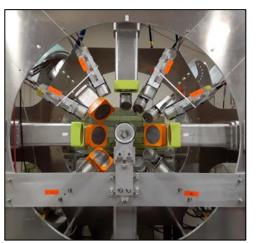
Nuclear Structure: New  $\gamma$ -ray Array at HI $\gamma$ S:
