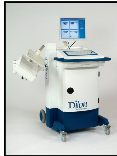
Compact gamma camera for breast cancer detection
