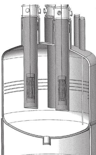
The concept for LEGEND-1000 showing a number of the deployments Ge detectors. This cut-away view shows three of five 200-kg groupings of Ge.
