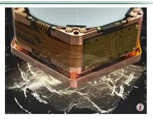
Naturally occurring radiation produced by environmental radioactive materials and cosmic rays is enough to limit the useful lifetime of superconducting qubit state to just a few milliseconds... Identifying ionizing radiation as a dominant source of excess quasiparticles... is a first step towards developing to mitigate its impact on superconducting circuits, including those used for quantum computation and quantum sensing.
