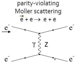
In MOLLER, polarized electrons are scattered of unpolarized electrons. The amount of parity violation due to interference of the two possible exchange mechanisms ( $\gamma$  or Z) is <u>precisely</u> predictable in QED. (No messy quarks or color charge, or QCD to worry about, only quantum electrodynamics). The theory is so "clean" that like the g-2 approach, If the level of parity violation is greater than expected, a new particle must be the source of the discrepancy.
