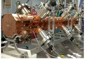
Figure S4: (Left) Centurion<sup>™</sup> Mk1 system being loaded into a van for transport to an off-site demonstration >1000 miles away. (Right) The compact RFQ LINAC itself (shown assembled with Starfire's patent-pending RF power injectors) is approximately 4' long and can be modified for energies between 1—5 MeV.
