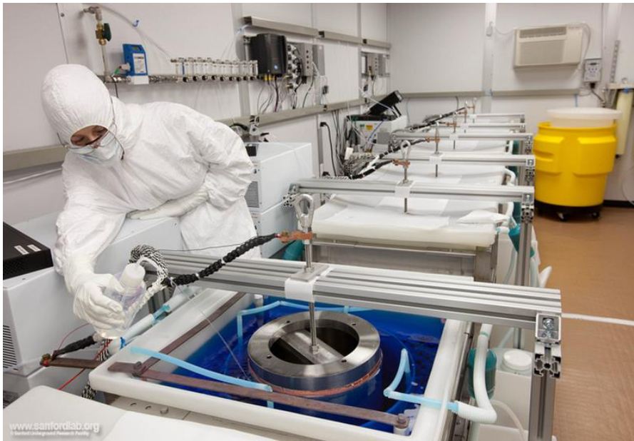
Mandrel insertion in MJD electroforming lab
