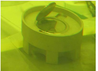
Open target in a hot cell showing Th "pie-slices" Target cut in "pieslices" to facilitate DOT Type A shipping
