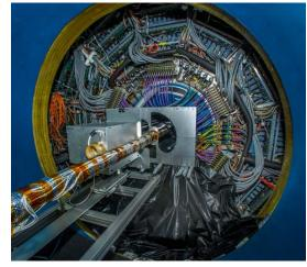
Heavy Flavor Tracker installed in STAR - ready for RHIC Run 14
