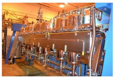
Cryomodule components at ATLAS (ANL)
