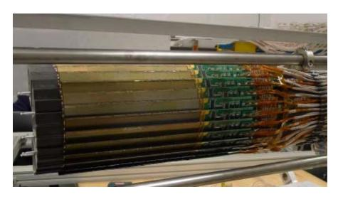
The recently completed STAR Heavy Flavor Tracker to enable measurement of heavy quarks
