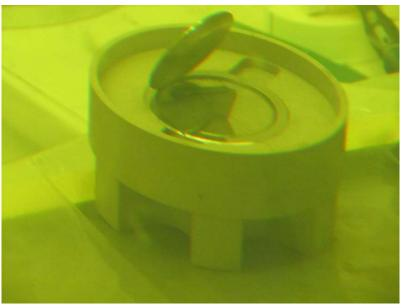
Open target in a hot cell showing Th "pie-slices" Target cut in "pieslices" to facilitate DOT Type A shipping
