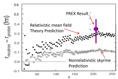
This result provides model-independent confirmation of the **existence of a neutron skin** relevant for neutron star calculations. Follow-up planned to reduce uncertainty by factor of 3 and pin down symmetry energy in EOS
