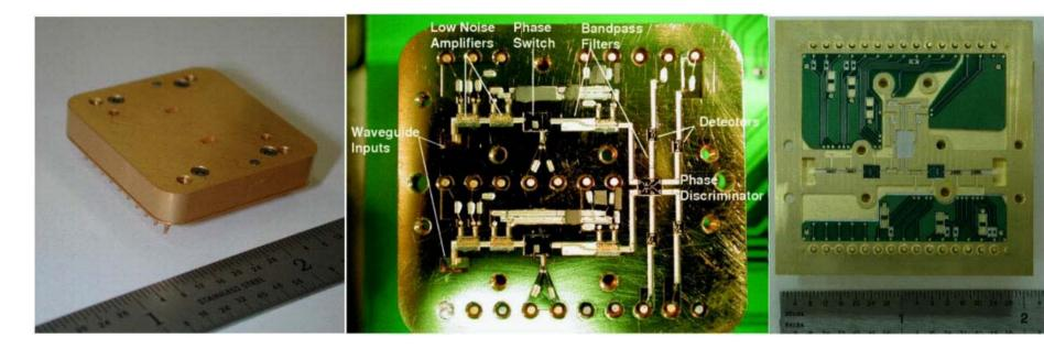
Left: Photograph of a prototype HEMT polarimeter with cover on and input waveguides shown. Center: The complete 90 GHz Q/U module shown with cover off. Right: The 40 GHz Q/U module shown with lid off. Photographs courtesy of Todd Gaier.
