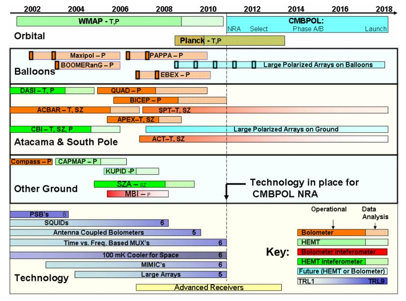
Schematic timeline of research programs observing CMB small-scale temperature fluctuations, CMB polarization, and the Sunyaev-Zel'dovich effect. The projects included in technology development are needed for ground-based, balloon and space
