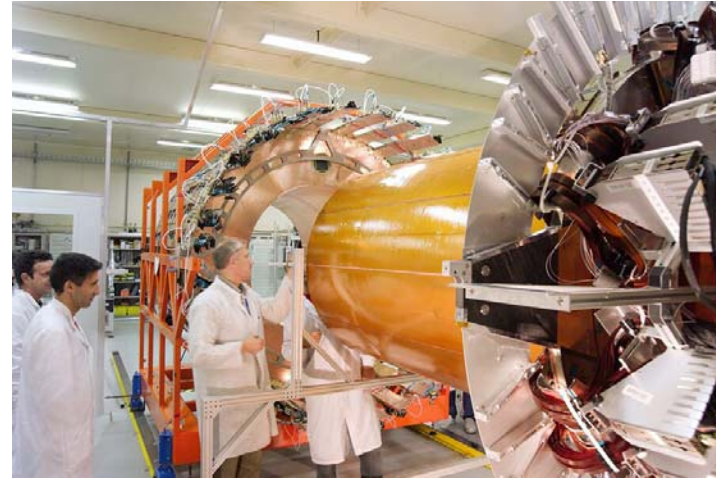
SCT End Cap C being inserted in TRT End Cap C
