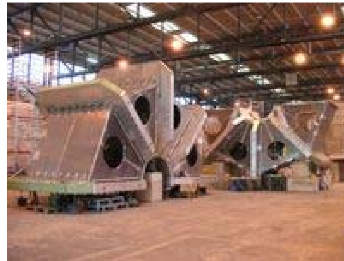
Two halves of End Cap Toroid C (ECT-C) cold masses under assembly in B180
