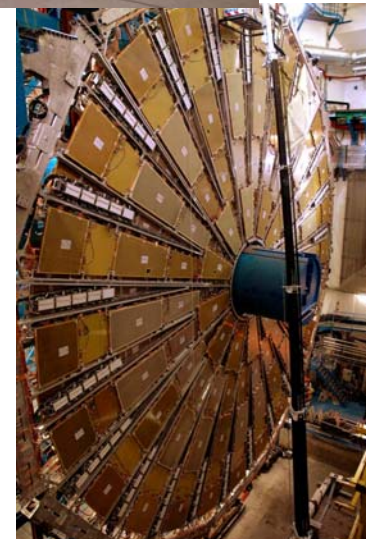
First of 6 TGC wheels installed in detector
