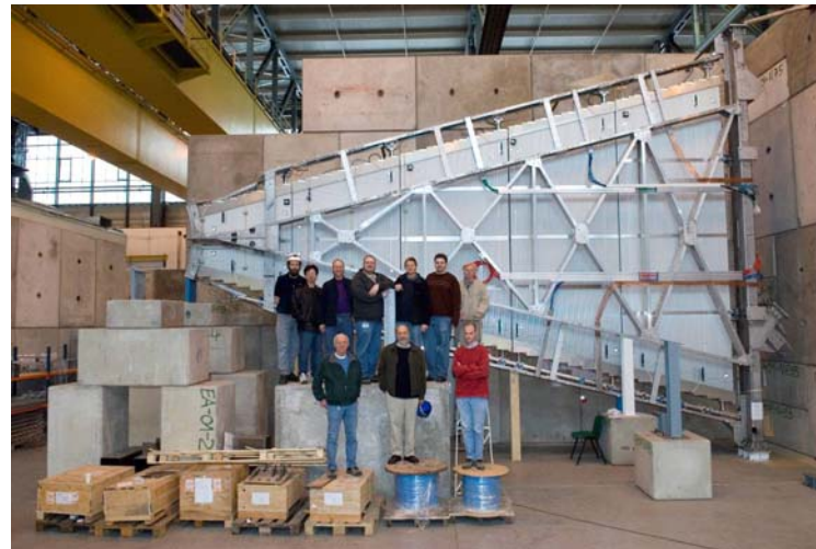
One of 32 MDT Big Wheel sectors ready for installation
