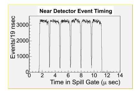
Beam arrives in 10  $\mu$ s batches
