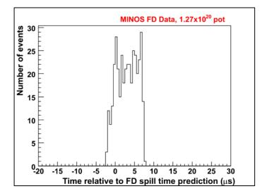
Far Detector triggers on spill time (50 μs window), also activity triggers
