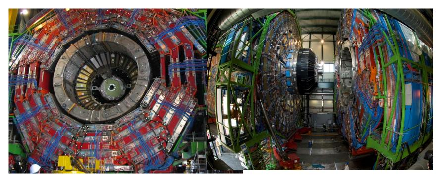
Goals were to test magnet to 4T and to read out each CMS subsystem – jointly – with cosmic ray muons. Note Tracker, EB, HB installed in magnet coil, MB chambers, ME CSC, HE.
