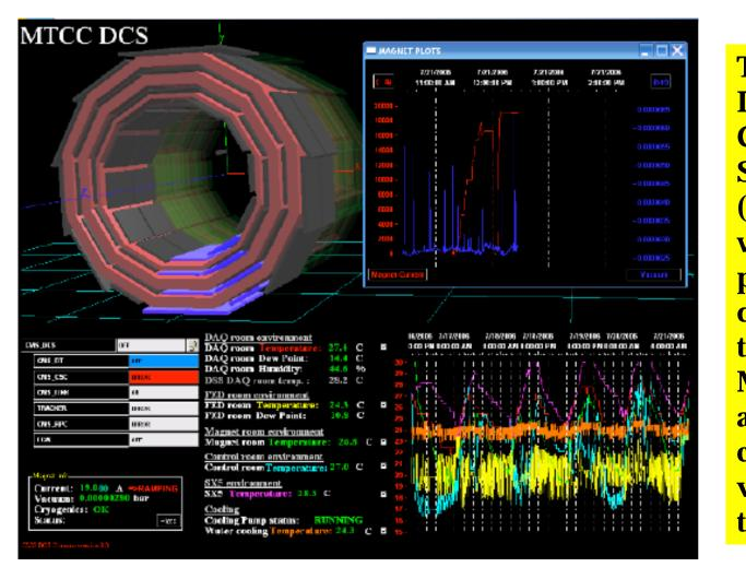
The **Detector Control System** (DCS) was in place during the MTCC and checked voltages, temps, etc.
