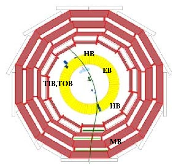
**Test of CMS** magnet at 4T. All **CMS subsystems** logged in global **DAQ** and synchronized. This is a major milestone on the way to CMS data taking. Muons can be used to cross check the HB and HE calibration and to align the muon chambers.
