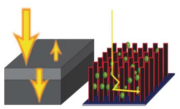
Al<sub>2</sub>O<sub>3</sub> nanoparticles reflect light towards Si wire arrays
