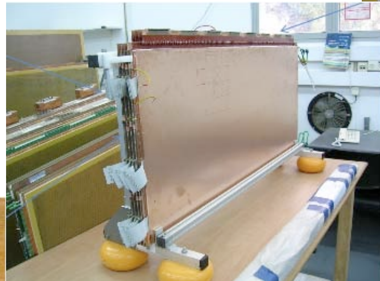
Fine strip Thin Gap Chambers
