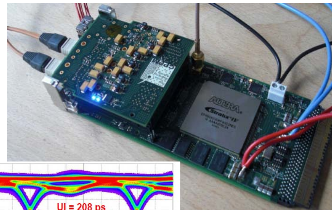
Eye-diagram from one channel @ 4.8 Gbit/s
