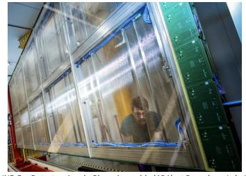
DUNE Far Detector Anode Plane Assembly (APA) at Daresbury Lab, UK, to be installed at CERN in NPO4, Horizontal Drift ProtoDUNE Module 0
