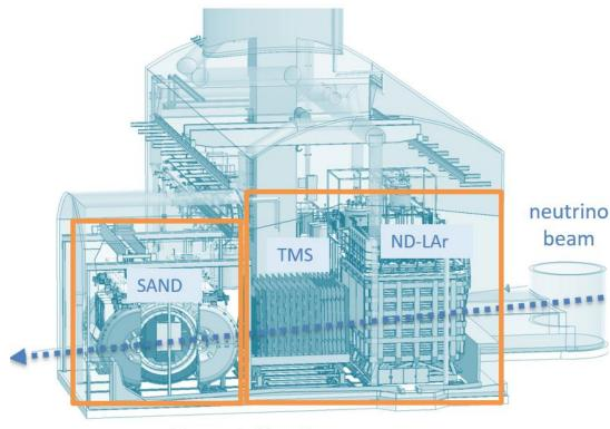
Two main Near Detector components: ND-LAr+TMS (moveable) and SAND (stationary)
