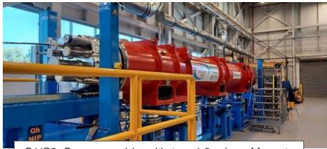
Q1/Q3 Cryo-assembly with two 4.2m long Magnets
