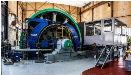
In March 2021, contractors completed major mechanical and electrical upgrades to the Ross Hoists at SURF (originally manufactured in the 1930s). Ross Hoists will power the excavation of 800 Ktons of waste rock and serve as the conveyance for people, materials and equipment underground.
