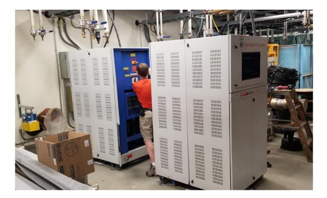
ECIL/BARC 7 kW 325 MHz amplifiers powered SSR1 cavities during beam testing at PIP2IT
