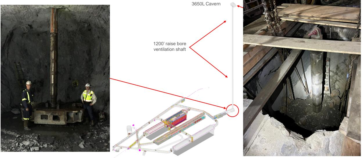
12' reamer head at breakthrough at 3650L Cavern – 4 Oct 2021
