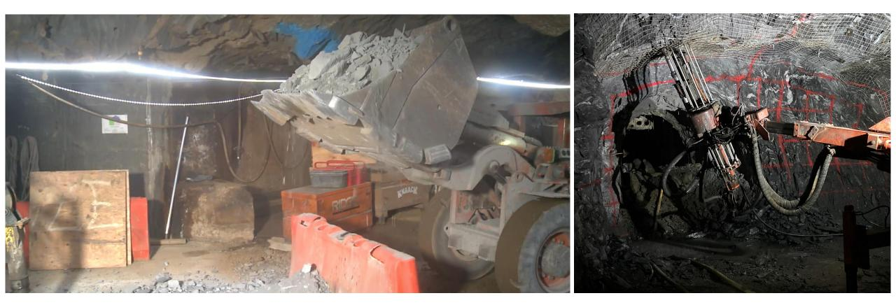
Moving "muck" to the ore bin, to be loaded in skip and moved to surface, crushed, and conveyed to the Open Cut
