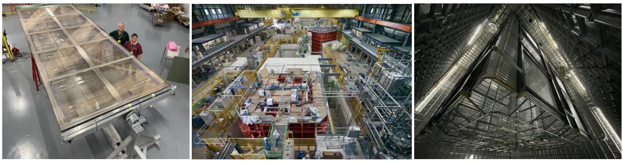
APAs for Module 0 ProtoDUNE being tested at Daresbury Laboratory, UK. One 2.3m x 6.3m APA is shown; UK to provide 130 APAs. NP-02 and NP-04 ProtoDUNE 8m x 8m x 8m detector prototypes at CERN.
