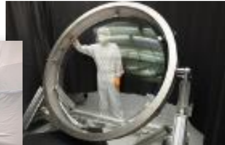
L1 Lens Coated and returned to AOS, L1 and L2 mounted
