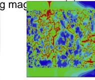
Predicted material damage and fracture development in dual-phase Ti3SiC2/SiC joints
