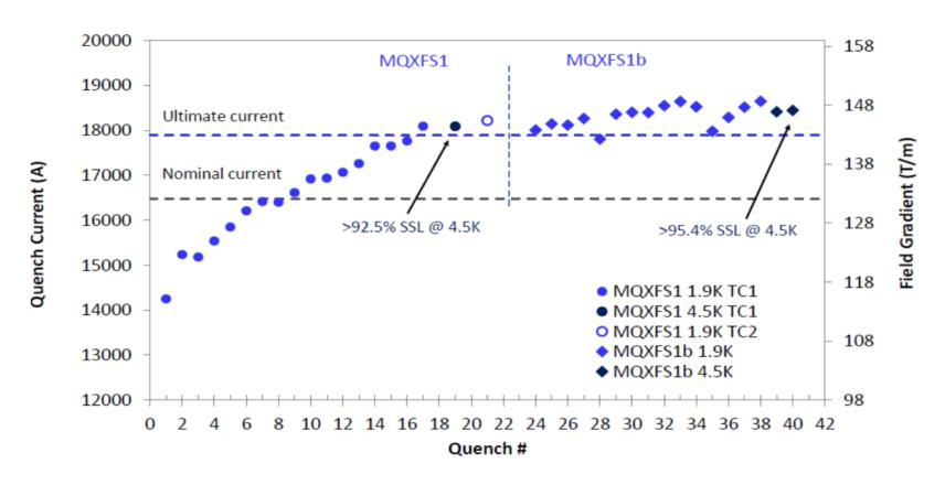
Highest quench current @1.9 K is 18649 A = 0.867 SSLHighest quench current @4.5 K is 18447 A = 0.958 SSL (actual T=4.66 K)
