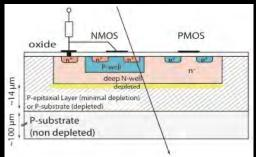
HV process, 10 - 15 μm depletion region under deep N-well
