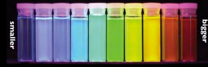
Wavelength shifting through Quantum Dots
