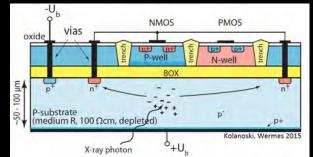
• Fully depleted or HV process
