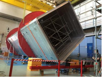
ICARUS cold vessel and new PMTs at CERN
