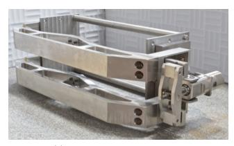
Double-Lever tuner prototype
