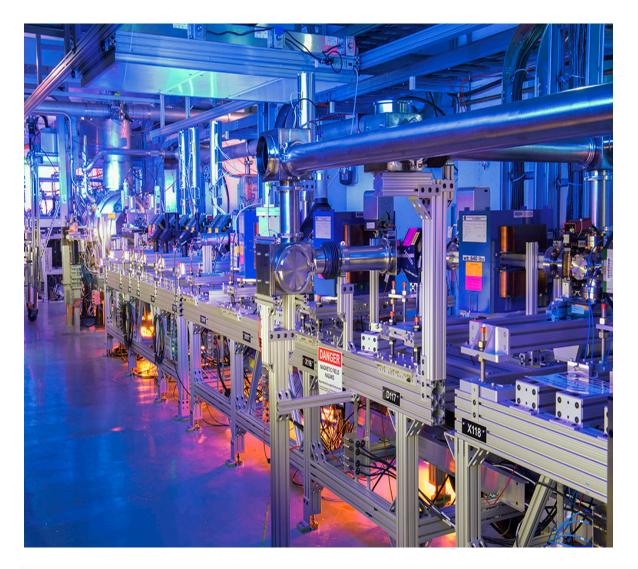
On Friday morning, March 27 first beam was delivered. We were able to deliver a 20 MeV electron beam from the **IOTA-Injector** photocathode, through a 1 m long SRF booster cavity CC2, and all the way to the beam dump, in front of the SRF Cryomodule 2.
