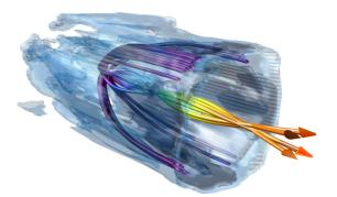
Figure 1. Computer simulation shows electrons being trapped and accelerated in a "bubble" (blue-grey cuplike structure) from a laser wakefield accelerator. Particle tracks are also shown for electrons successfully trapped by the wake. The color of the tracks, from purple to red, shows the increase in electron energy along the track. (Image: W.B. Mori and L.O. Silva)
