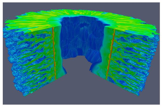
**Figure 2-3.** A simulation of a nested wire array Z-pinch using a 3-D MHD code with 700 million computational elements. (J. Chittenden, Imperial College, London)
