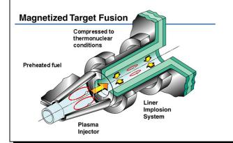
a) The 10-microsecond variant of MIF utilizes the magnetic pressure produced by a 12-MA current to implode a cylindrical metallic liner (green). A magnetically confined plasma formed outside the liner (red ellipses to the left of liner) is injected into the liner as it is imploding. This plasma is compressed and heated to fusion conditions by the time the imploding liner stagnates against the plasma. (AFRL/LANL collaboration)
