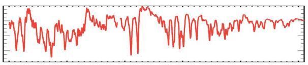
Figure 2. Transmitted intensity versus wavelength - transmission spectrum for iron heated to 1.8 million degrees. The peaks and valleys of the data carry a wealth of information about the different electronic states iron atoms take in the plasma, such as in the interior of a star. This type of data can be used to test quantum mechanical models of iron opacity.
