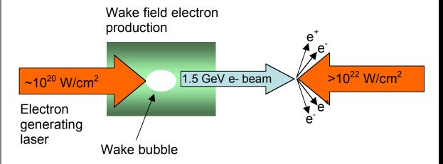
Conceptual diagram of an all-laser-based experiment to study nonlinear QED at and beyond the Schwinger field. It requires splitting an intense laser into two beams, one that produces the dense electron cloud (right-moving), and one that interacts with them (left-moving). Their collision produces acceleration of the electrons that break down the vacuum and create a multitude of pairs.
