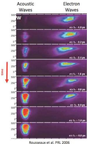
**Figure 3-2.** Studies using snapshots of light scattered from electron plasma waves and ion acoustic waves driven by intense laser beams show that the electron wave is dying out while the acoustic wave is growing. This is an indication that the laser light is mediating the energy transfer between the waves. Such processes can one day be developed to control the flow of energy in HED plasmas.
