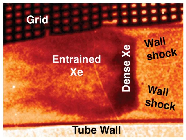
**Figure 4-2.** An X-ray radiograph of a radiative shock imaged 14 nanoseconds after high-energy laser beams irradiated a thin beryllium disk. The shock is moving to the right in this image into the unshocked xenon gas. The xenon gas is swept up by the shock, creating the dark structure in the image.
