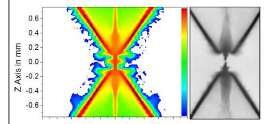
Figure 2. At left, a slice through a 3-D simulation of an imploding X-pinch reveals the formation of a narrow plasma column where the wires cross. At right, a flash of X-rays from one X-pinch (not shown) is used to capture the instant when the center of a second X-pinch collapses to a few millionths of a meter. (Left image, Imperial College; right image, Cornell University)
