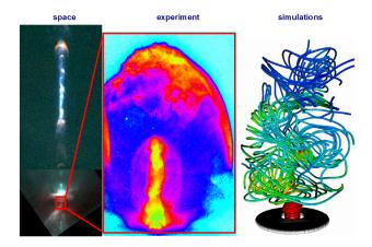
Figure 2-2. Scaled experiments (center) combined with high-performance computer simulations that include magnetic field evolution (right) aid in understanding the nature of launch regions of astrophysical jets (left) that are too small to be clearly observed. The launch region is represented by just 2 cm in the experiment, but the physics at work is believed to be the same as in solar-system-sized jets from young stars. (NASA/Imperial College/Paris Observatoire)
