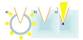
Figure 1. a) In a fast-ignition target, the outer shell (blue) is irradiated by a compression driver (yellow) to b) create a dense fuel core, which is then c) ignited by a picosecond laser (yellow) to create electrons (blue). The electrons propagate into the dense core and create an ignition spark (red).
